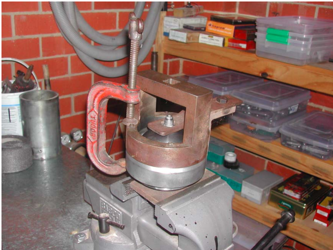
The fixture to undo the spheres. The clamp is to hold the 'spanner' in place. There were two methods of sealing the charging valve involving the shape of the projection. One was sealed with an 'O' ring and the other with a plastic ball which was crushed into the charging hole when the cap was screwed on. Practice has been to use the ball on both to ensure a seal.
