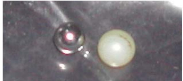
The steel ball on the left goes in the seat inside the sphere and is held in place by a small spring and even smaller circlip. The plastic ball on the right is forced into the outer end of the charging valve and topped with the charging cap after charging.
