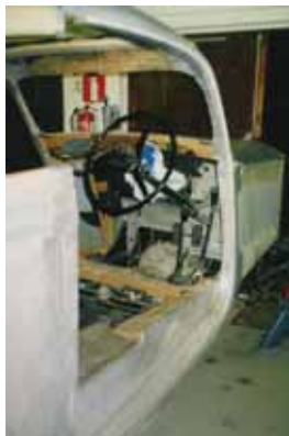
The making of the framework of the right hand door, its frames and fitting in place.
