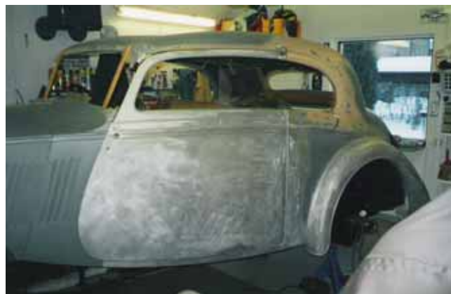
Left hand door in its proper place, wooden sticks acts as A-pillars.
