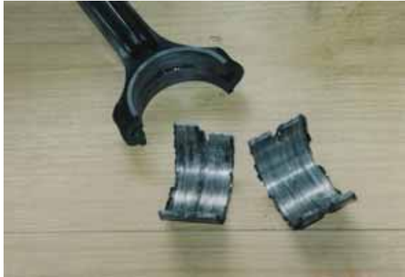
The lower bearing of the 5 th cylinder connecting rod and oil sump removed
