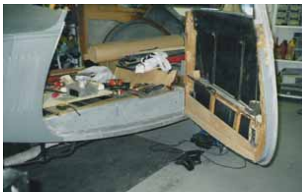
The left sill welded ready
