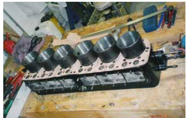
Head, and cylinder group after machining
