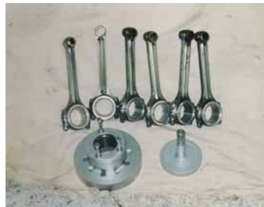
Connecting rods with new bearings waiting for engine assy. At the bottom home made fixtures to make sure that white metal bearings at the both ends of connecting rods were machined parallelly .
