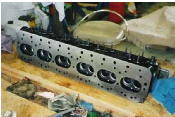
Head, and cylinder group after machining
