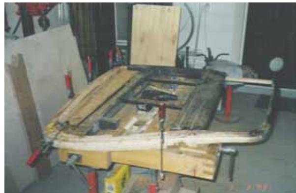
The making of the framework of the right hand door, its frames and fitting in place.
