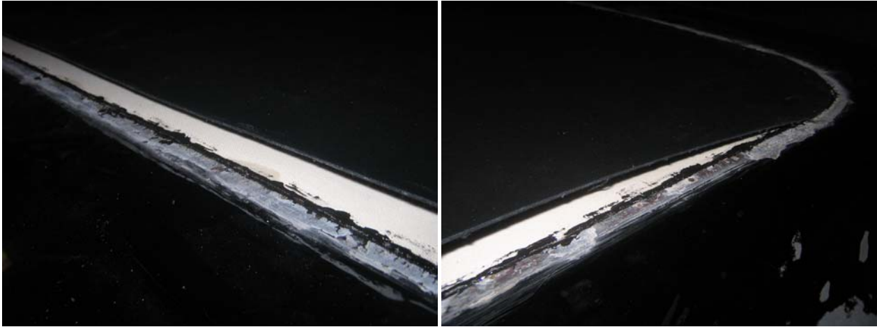
Leathercloth should completely cover cotton and almost meet the aluminium body.
