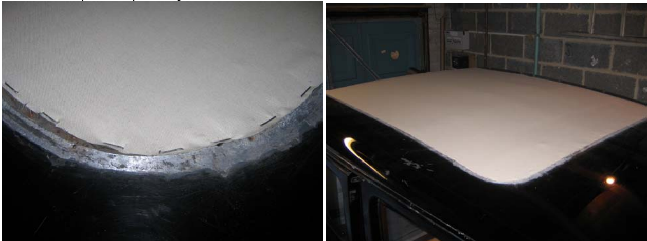
Cotton sheeting should just fall short of the aluminium bodywork. Finished cotton should appear smooth and tight.
