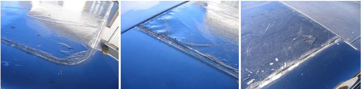
Above with brass strip removed – note deterioration of the leathercloth.
