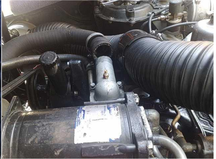
A new gasket installed and back in place ready for the upper hose reconnection and wiring to be put into place.
