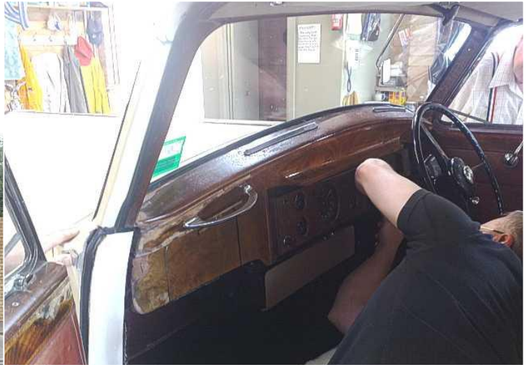
Neil gets stuck into removing the centre dash panel to get access to the fuel gauge on his Silver Wraith.
