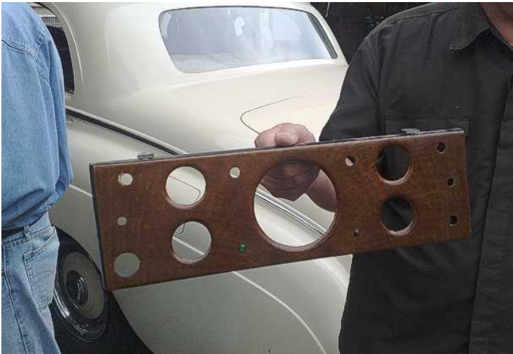
Appearances can deceive. The walnut veneer is mounted on an aluminium base
