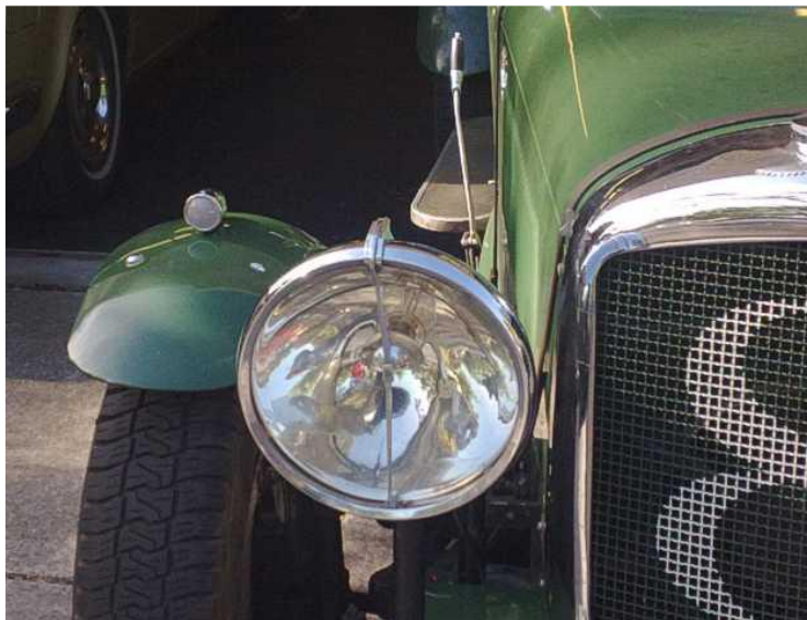
Sidelights installed of the wheel arches to compliment the R100 headlamps
