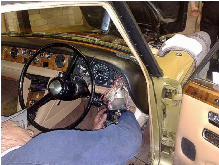
Connecting the electrics to an existing fusible wiring circuit
