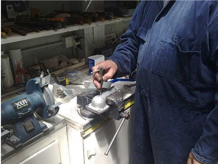
The thermostat inlet housing was 'very carefully' secured in the vice before being drilled and tapped to accept the temperature sensor unit
