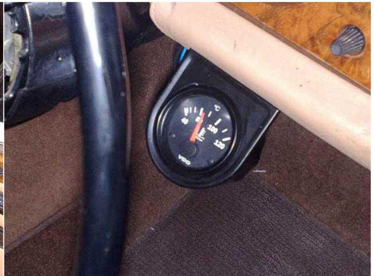
The gauge was mounted discreetly so that only the driver could easily view the temperature
