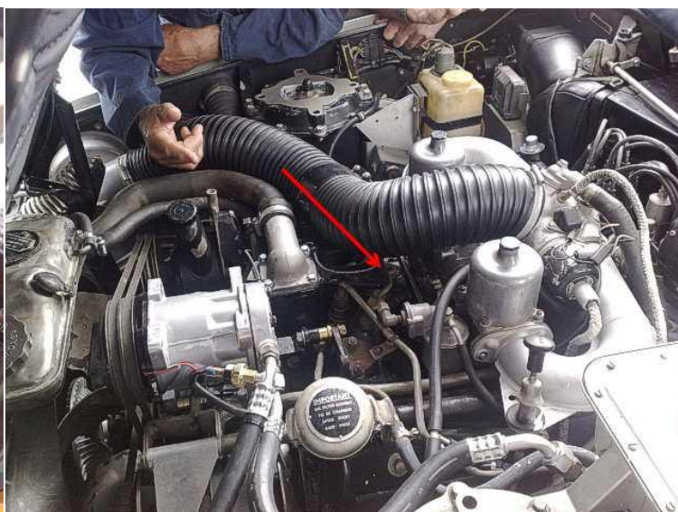
The red arrow points to the position of a coolant plug situated on the inlet manifold casting which is the ideal spot to fit the sender unit for the temperature gauge.
